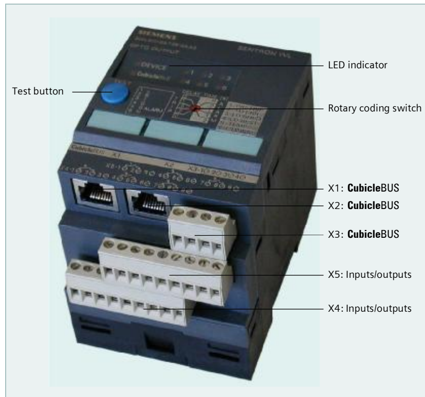
Fig. 2-8 All external CubicleBUS modules have the same housing. The CubicleBUS can be connected to X1 and X2 with an RJ45 plug or a terminal connection made to X3. This depends on whether a COM15 module is available.
