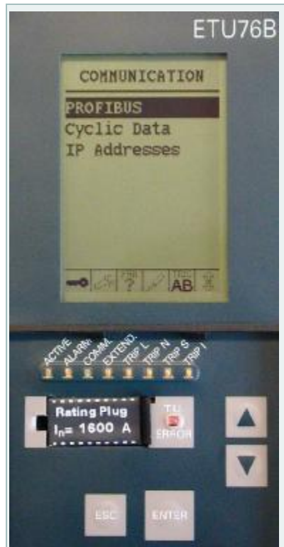
Fig. 4-7 The ETU76B display also enables you to change the communication parameters
