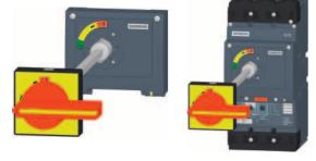
The rotary operating mechanism makes possible to govern the circuit breaker by pivoting knob, e.g. to switch machines on and off. Modular conception of operating mechanisms makes possible simple mounting on the switching unit (also additionally) after the accessory compartment cover is removed. A fixed motor is possible to seal. The operating mechanism and its accessories is ordered separately according to your choice (see page 3/6).
