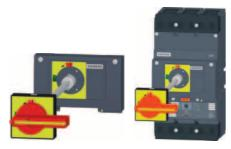
The rotary operating mechanism makes possible to govern the circuit breaker by pivoting lever, e.g. to switch machines on and off. Modular conception of drives makes possible simple mounting on the switching unit (also additionally) after the accessory compartment cover is removed. A fixed motor is possible to seal. The drive and its accessories is ordered separately according to your choice (see page 4/6).
