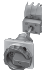
3LD2 213-0TK5 switch for floor mounting with rotary operating mechanism and defeatable door coupling
