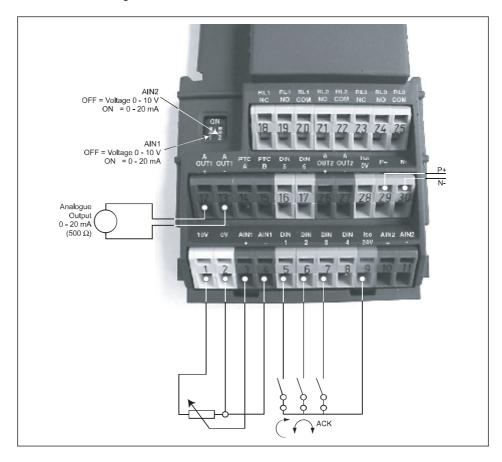
Figure 3-4 Basic operation with SDP
