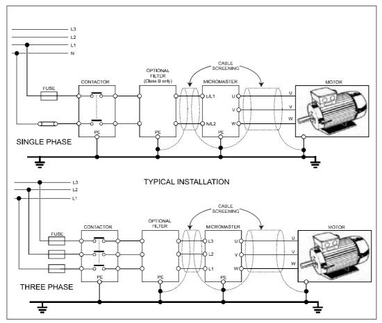
Figure 2-6 Motor and Power Connections
