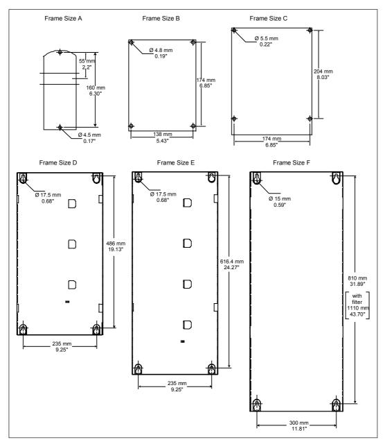
Figure 2-4 Drill pattern for MICROMASTER 440
