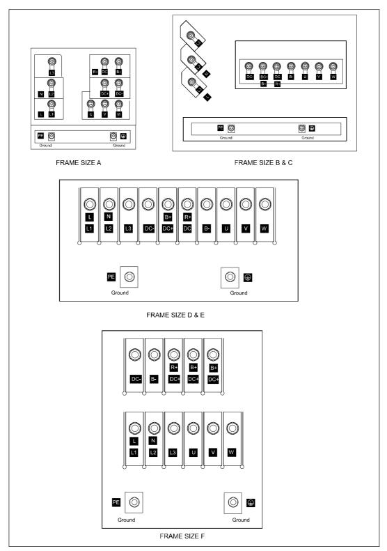
Figure 2-5 MICROMASTER 440 Connection Terminals
