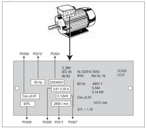
Figure 3-7 Typical Motor Rating Plate Example
