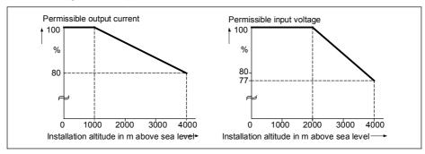
Figure 2-3 Installation altitude
