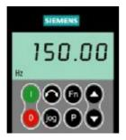
You can alter parameter values via the BOP. To set parameters on this panel, you must remove the SDP and attach the BOP (see Appendix 0).
