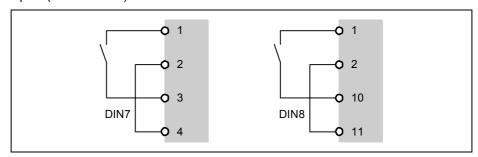
Figure 3-2 Configuration of the analogue input as a digital input
