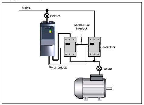
Figure 4-1 Bypass circuit
