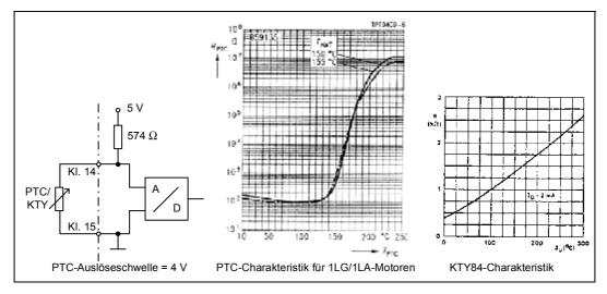
Figure 3-9 Thermal overload protection
