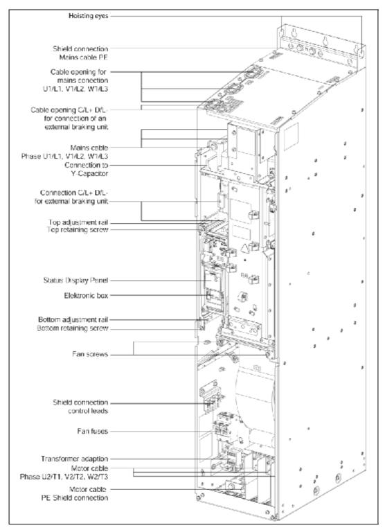
Figure 2-10 MICROMASTER 430 connection drawing – frame size GX
