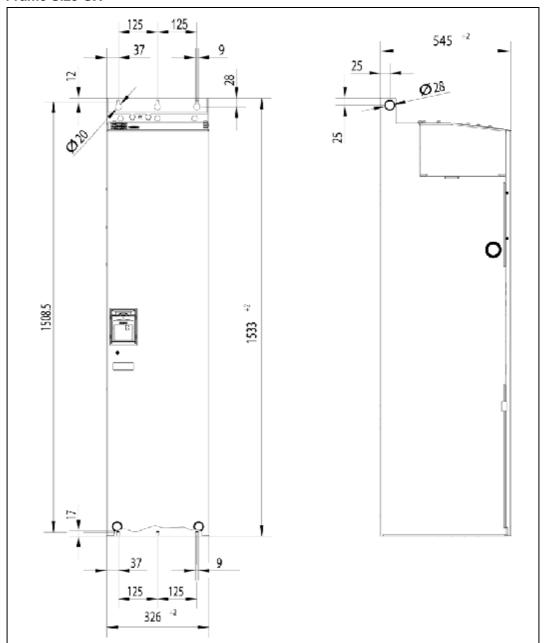
Figure 2-6 Installation dimensions for MICROMASTER 430 Frame size GX
