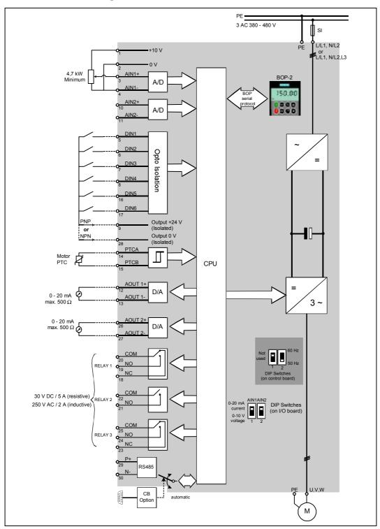
Figure 3-1 Inverter block diagram
