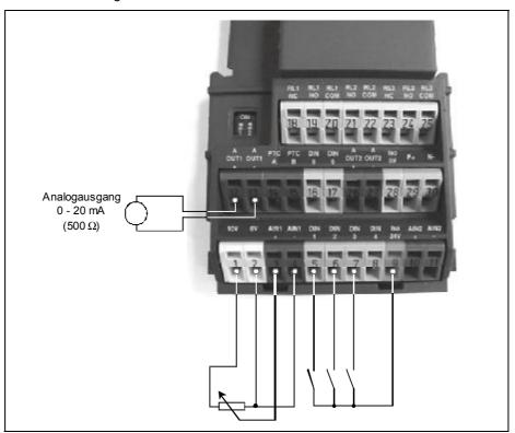
Figure 3-5 Basic operation with SDP
