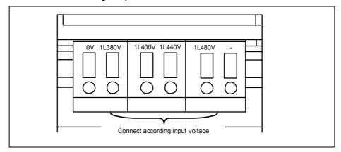
Figure 2-12 Adaptation of fan voltage
