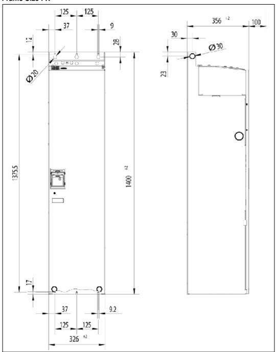
Figure 2-5 Installation dimensions for MICROMASTER 430 Frame size FX
