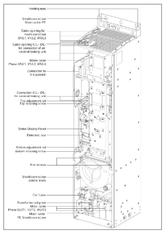
Figure 2-9 MICROMASTER 430 connection drawing – frame size FX
