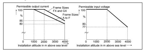
Figure 2-3 Installation altitude
