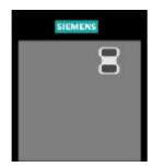
The SDP has two LEDs on the front which display the current operating status of the inverter (see Section 6.1).
