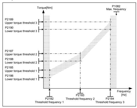
Figure 4-2 Belt Failure Detection
