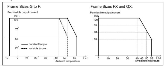
Figure 2-2 Ambient operating temperature
