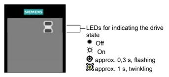
Table 6-1 Inverter conditions indicated by the LEDs on the SDP
