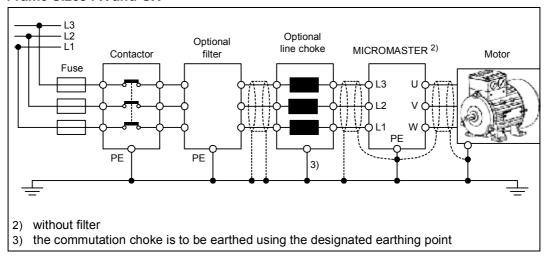
Figure 2-11 Motor and Power Connections
