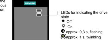
Table 6-1 Inverter conditions indicated by the LEDs on the SDP
