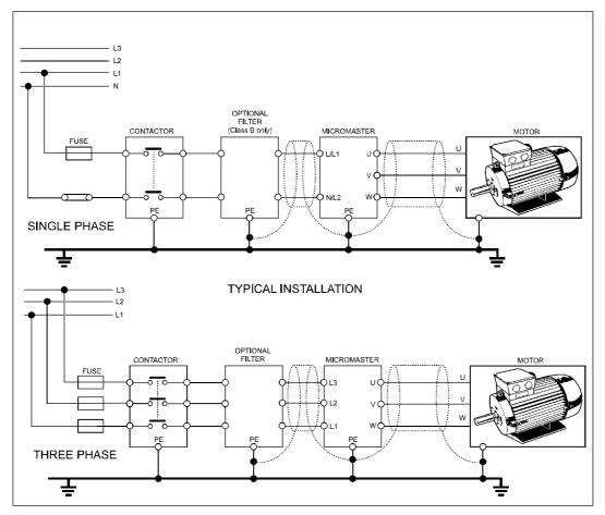
Figure 2-6 Motor and Power Connections
