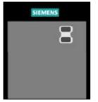
The SDP has two LEDs on the front which display the current operating status of the inverter (see Section 6.1).
