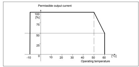
Figure 2-2 Ambient operating temperature
