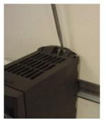
1. Fit the inverter to the rail using the upper rail latch.
