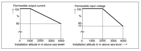
Figure 2-3 Installation altitude
