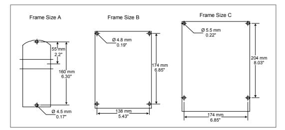
Figure 2-4 Drill pattern for MICROMASTER 420
