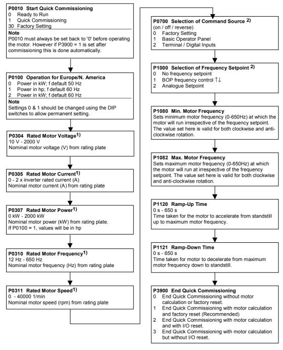
1) Motor-specific parameters – see motor rating plate.
