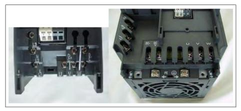
Figure 2-5 MICROMASTER 420 connection terminals
