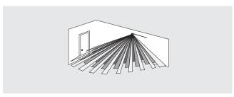
The sensing levels of the 2.20 m lens arranged from the top to the bottom.
