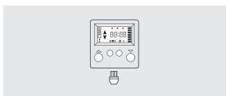
The sun sensor cable is connected by plugging the plug of the sensor into the socket of the Comfort shutter/blind clock.
