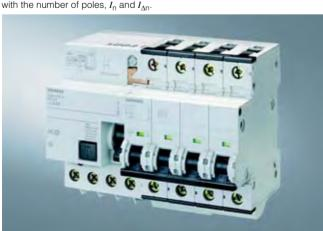
The two components are simply plugged together without the need for any tools. After the connecting screws of the conductor connection between the RC unit and the miniature circuit-breaker have been tightened, the two devices form an RCBO.
