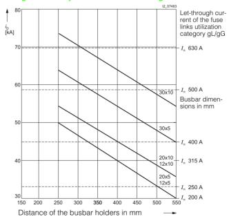
iD: Let-through values (kA) of the LV HRC fuse links, utilization category gL/gG with rated current 200 Å to 630 Å for prospective short-circuit current  $I_{\rm D} = 120 \, \rm kA.$
