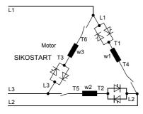
Fig. 23 : Proper Inside Delta Wiring Connection
