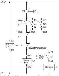
Fig. 9 : Typical Overtemperature Switch Wiring
