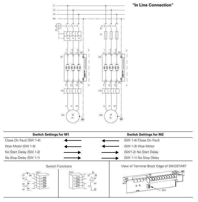
Fig. 12 : Power wiring for motors, wired "In Line", in a vented enclosure (circuit breaker or fusible disconnect)
