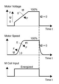
Fig. 5 : Voltage and time curves for soft start with coast to stop
