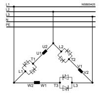
Rated Current  $I_e$  Equals Approx. 58 % of Motor Rated Current  $I_n$ 6 Leads to the Motor (Like for Wye-Delta Starters)
