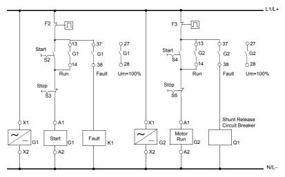
Fig. 17 : Control wiring for motors, wired "Inside Delta" in a vented enclosure, with fusible disconnect and isolation contactor, and shunt release.
