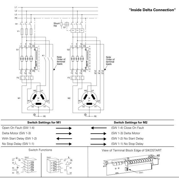
Fig. 16 : Power wiring for motors, wired "Inside Delta" in a vented enclosure, with fusible disconnect and isolation contactor, and shunt release.
