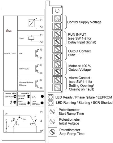
Fig. 3 : SIKOSTART Control Terminals with Us DC 24 V
