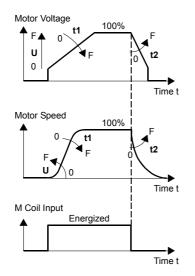
Fig. 6 : Voltage and Speed Curves for Soft Start with Soft Stop
